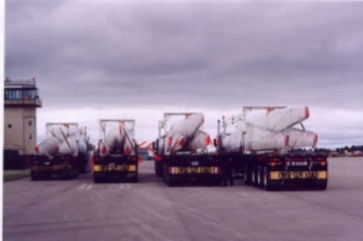
Figure 1 - Transport of Blade Sets
